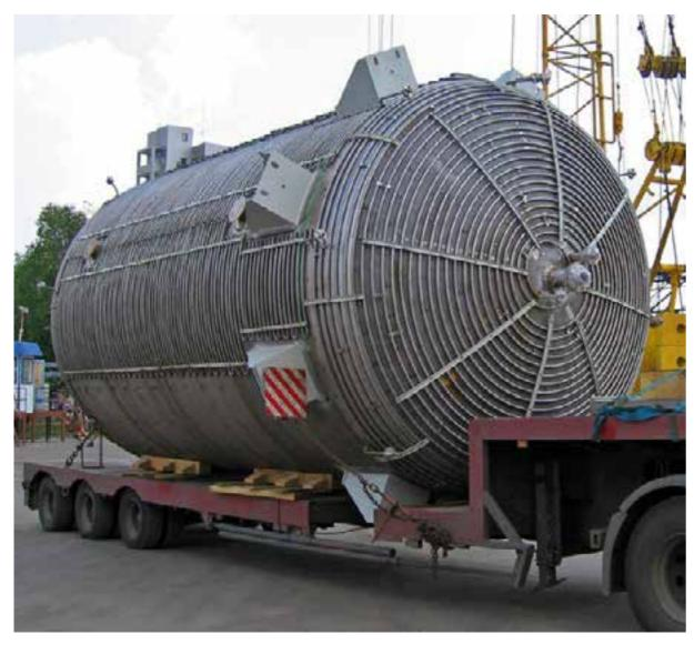
ZAVKOM produces polymerizers for polymer solution processes. Polymerizers are vertical cylinder apparatus equipped with branching pipes for raw charging, catalyst agent feed and subsequient reaction mass extraction. Polymerizers may be equipped with the cooling jacket, cylindric-shaped build-in cooling internal barrel, agitator, scraper-type agitator, internal heat exchangers.
