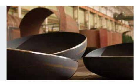
In 2004, ZAVKOM using the equipment of «Schleifstein» company (press for accelerating punching, Edge-bending machine) mastered the serial production of heads and bottoms for capacitive equipment by cold stamping and rolling method with internal diameter from 800 mm to 7,200 mm and wall thickness from 3 mm to 30 mm.
